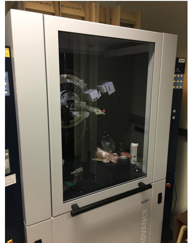
Image: Automated Bruker D8 Advance DaVinci PXRD w/LYNXEYE XE-T Detector leased by Asha at UCSD
