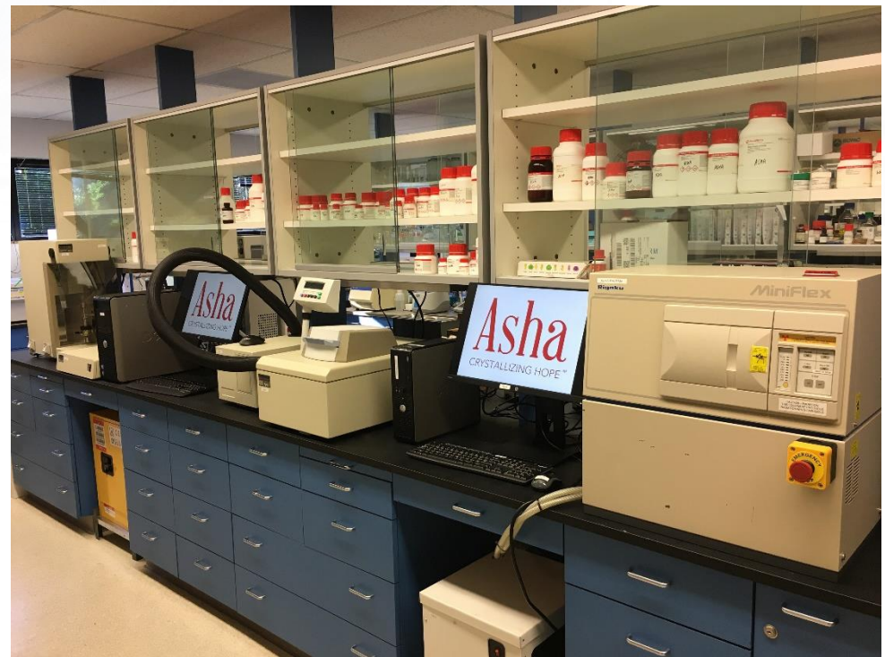
Image: Asha's Fully Equipped Solid State Lab with PXRD, DSC & TGA Instruments Shown
